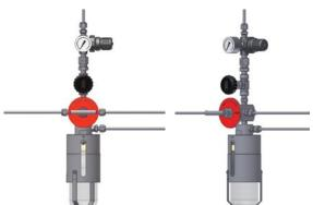
The ability to purge the needle assembly, both before and after sampling, ensures there is no residue build up in the needle assembly after retrieval of a representative, contamination free sample. The DPM type of sampler in an inline needle purge configuration allows product to flow directly into the sampler via an inline sample valve.
