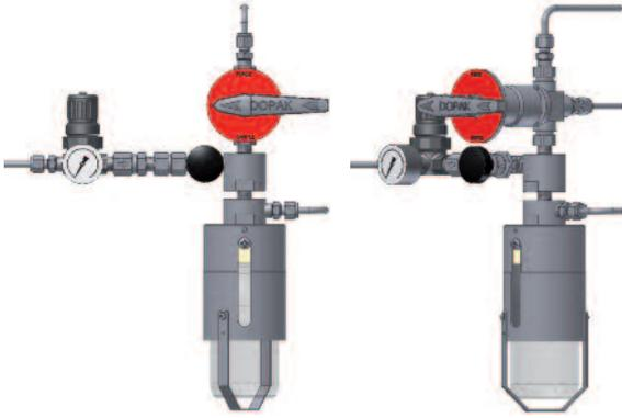
The ability to purge the sample point ensures optimal retrieval of a representative and contamination free sample. The DPM type sampler in system purge configuration allows product to flow continuously through the sampler ensuring a fresh sample and also allows to purge the needle assembly continuously before and after sampling.
