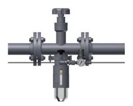
The ability to install the sampler directly in the process line ensures optimal retrieval of a representative, contamination free sample. The DPT type of sampler in continuous needle purge configuration allows the product to flow directly into the sampler via an in line sample valve and to purge the needle assembly continuously before and after sampling.
